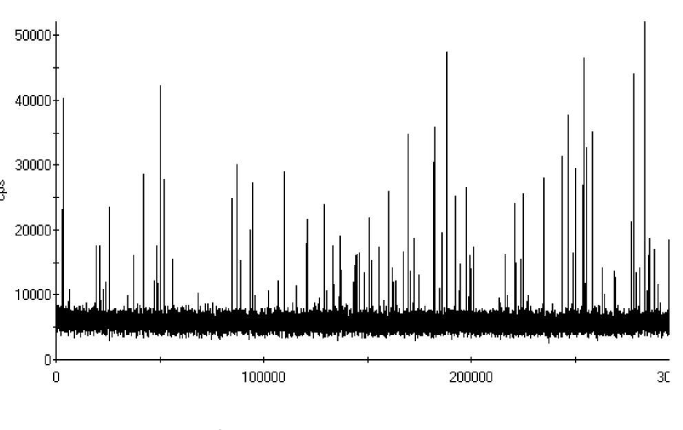
Example of raw single particle ICP-MS data of titanium spikes in a pool sample
