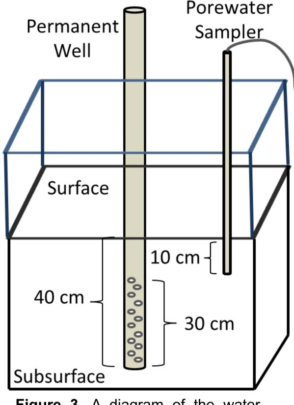
**Figure 3.** A diagram of the water sampling apparatus used for this investigation.
