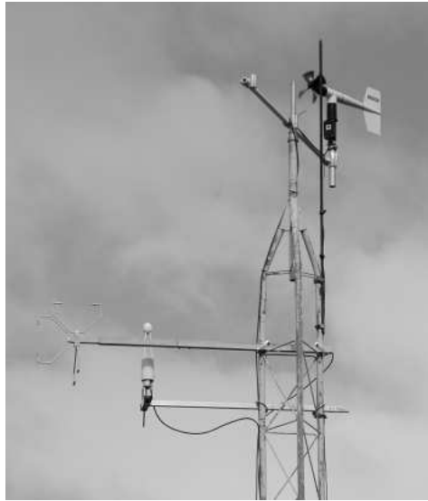
Figure 4.5: Eddy correlation equipment at the Lost Dutchman State Park (LDP) site. The sonic anemometer and infrared hygrometer booms extend to the left from the tower. The propeller anemometer is at the top of the tower.
