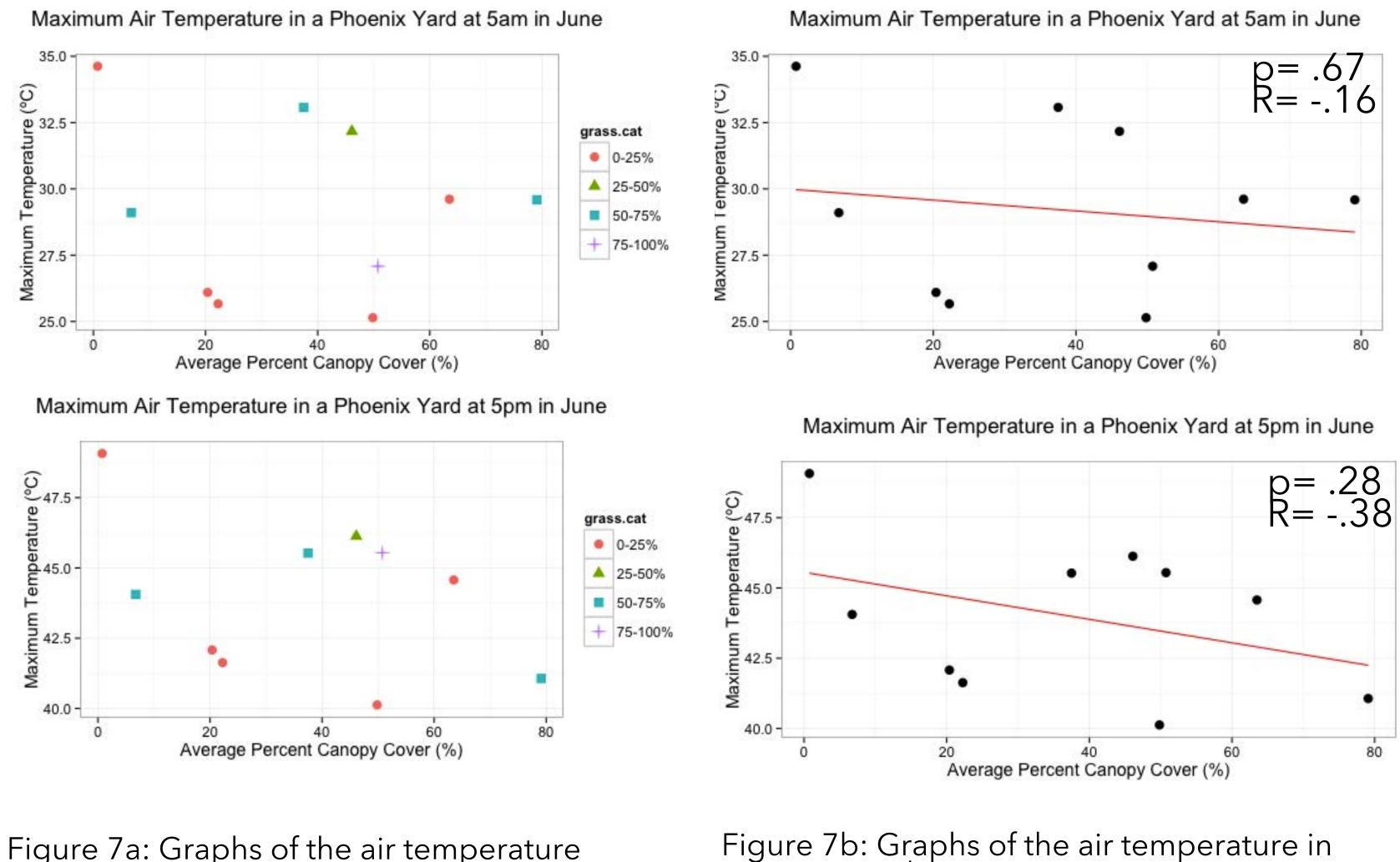
Figure 7a: Graphs of the air temperature in June versus the average percent canopy coverage at periods of low (5am) and high (5pm) wind speeds, with respect to the percentage of grass
