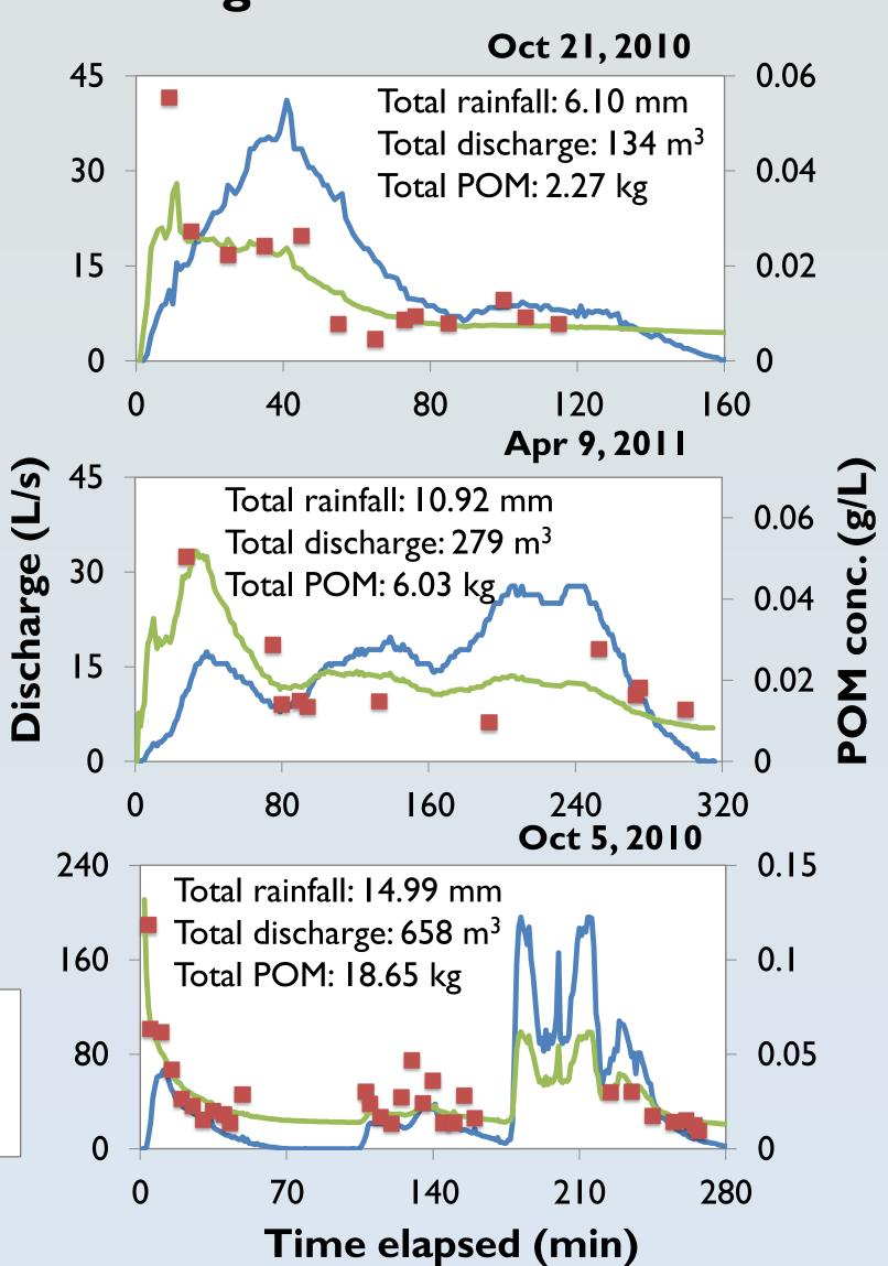
Street drainage: rapid transport of POM through the system, resulting in an exponential decline in POM concentration.
