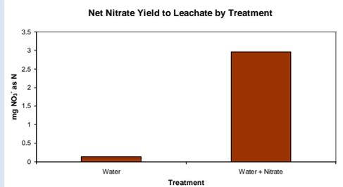
Figure 3: Addition of nitrate to water leaching through soil cores. In treatment 2, more nitrogen came out of the core than was put in. Even the cores receiving water alone (treatment 1) resulted in a positive yield in the leachate.
