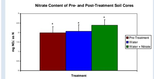
Figure 4: Amount of extractable nitrate from pre- and post-treatment soil cores. Error bars are standard errors. Note that there is no significant difference among treatment groups, i.e. addition of water, or water + nitrate, did not effect net nitrate content.
