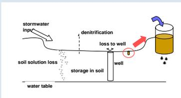
Figure 1: Graphical representation of a stormwater retention basin, showing major components and abstraction of soil cores.
