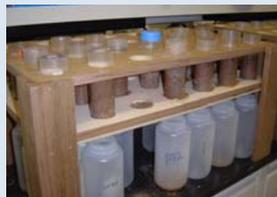
Figure 2: Laboratory setup of suspended soil cores with bottles beneath to collect leachate.
